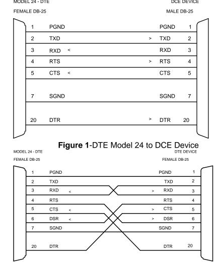
Figure 2-DTE Model 24 to DTE Device
